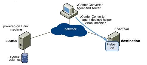
2 The helper virtual machine powers on, boots from the Linux image, connects to the source machine through SSH, and starts retrieving the selected data from the source. While you set up the conversion task, you can select which source volumes to be copied to the destination machine.
