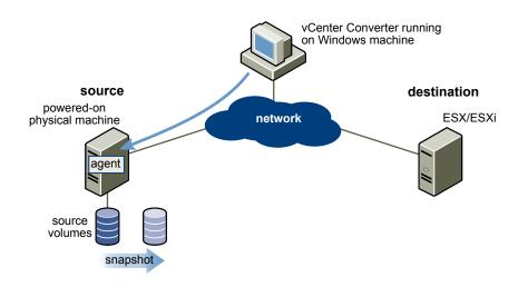
2 vCenter Converter prepares the virtual machine on the destination machine.
